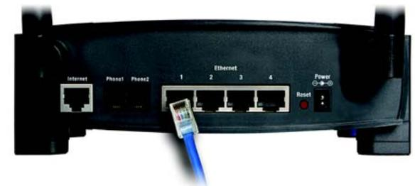
Figure 4-8: Connect the Other Router
