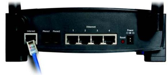
Figure 4-6: Connect the Broadband Modem
