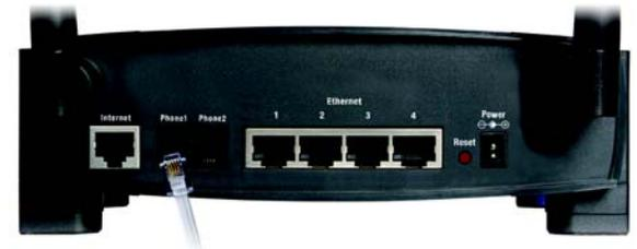
Figure 4-7: Connect a Telephone
