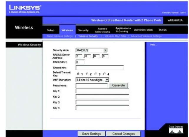
Figure 5-13: Wireless Tab - Wireless Security (RADIUS)
