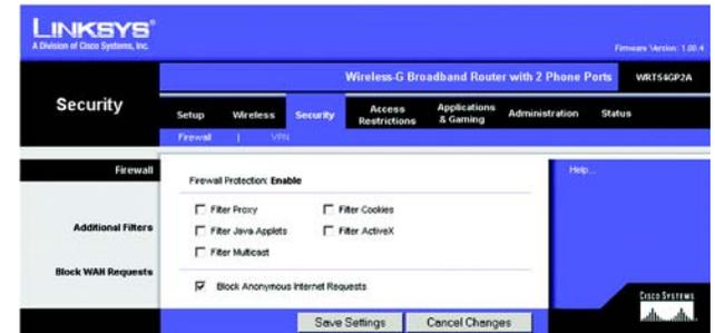
Figure 5-19: Security Tab - Firewall
