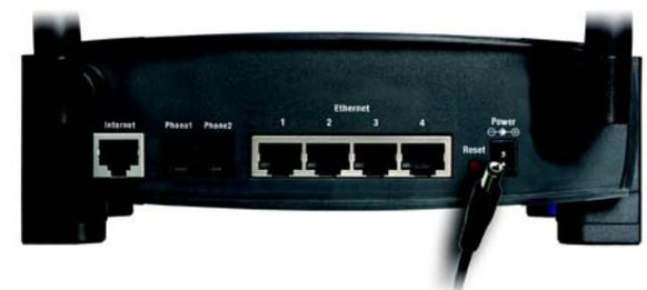
Figure 4-9: Connect the Power
