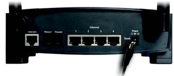
Figure 4-4: Connect the Power
