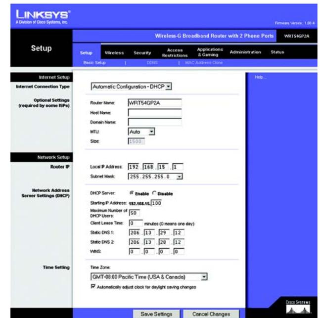
Figure 5-3: Setup Tab - Basic Setup - Automatic Configuration (DHCP)
