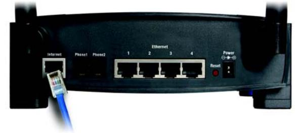
Figure 4-1: Connect the Broadband Modem
