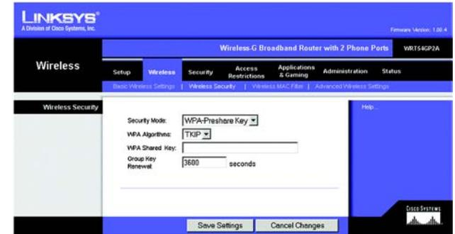
Figure 5-11: Wireless Tab - Wireless Security (WPA Pre-Shared Key)
