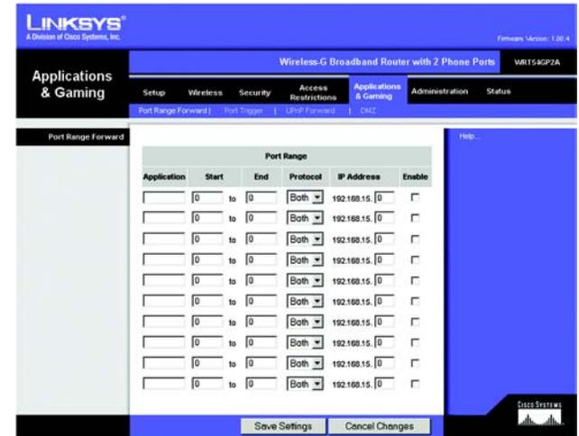
Figure 5-24: Applications & Gaming Tab - Port Range Forward
