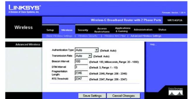
Figure 5-18: Wireless Tab - Advanced Wireless Settings
