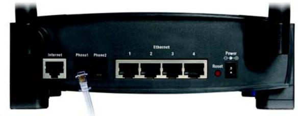
Figure 4-7: Connect a Telephone
