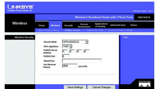
Figure 5-12: Wireless Tab - Wireless Security (WPA RADIUS)
