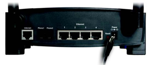
Figure 4-9: Connect the Power
