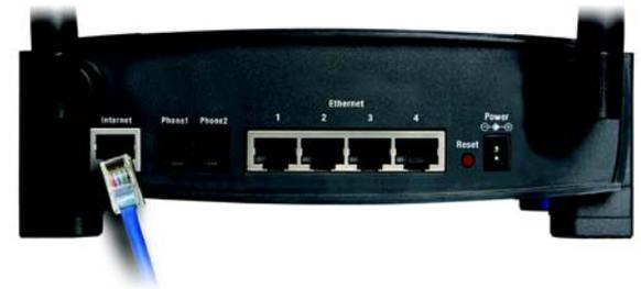
Figure 4-6: Connect the Broadband Modem
